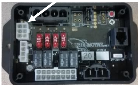
Data Link Harness plugs in here
