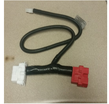
IDLE Data Link harness "T's" into OBDII connector.
