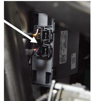
Charger gateway module with 8 & 12-pin connectors.
