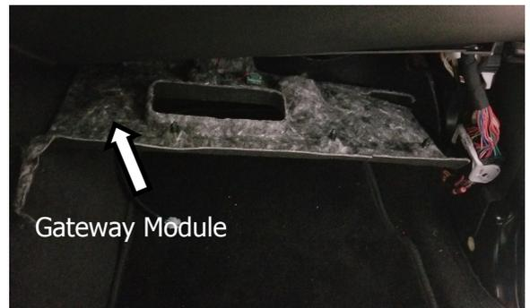
1. Locate the vehicle's Gateway module located on the left side of the glove box.
