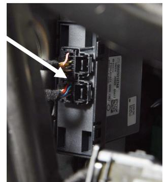
Durango gateway module with 8 & 12 pin connectors.
