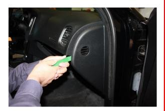
4. Remove the 8 screws around the perimeter of the glove box.
