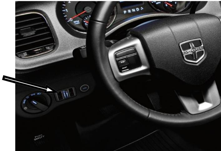
Rotate the left dimmer control to the extreme bottom OFF position. The interior lights will remain off when the doors are open, and the PIM will mute the driver door related chimes.
