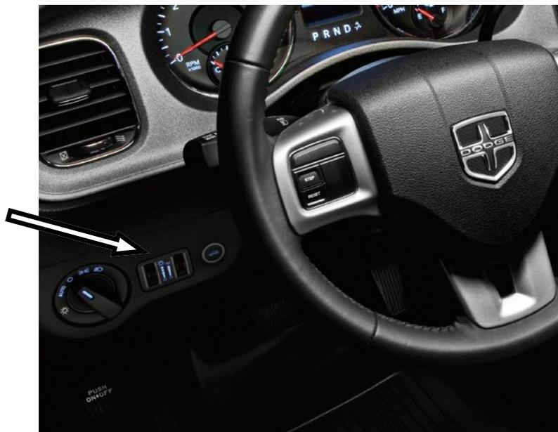
Rotate the left dimmer control to the extreme bottom OFF position. The interior lights will remain off when the doors are open.
