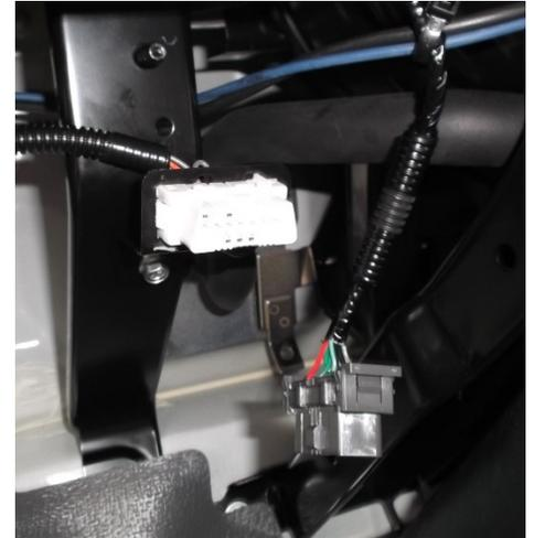
OEM OBDII bracket with White ITC950 connector installed, with Grey OEM connector in lower right
