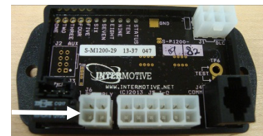
View from floor looking up at underside of transmission shifter PCB. Arrow points to the 2 pin Shift Lock Harness.
