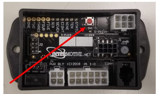
Press Test button 3X to enter Diag. Mode
