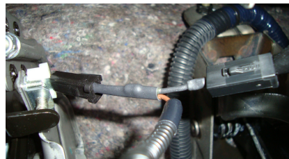
Park Brake connection behind pedal
