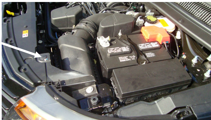
Location of plastic connector stub in place of OEM hood switch
