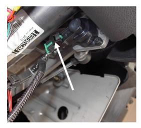
**Black 1-Pin Connector** – Disconnect the black, single-wire Chevrolet connector from the park brake switch (see photo). Plug the female side of the connector from the Brown wire on the ILIS main harness to the parking brake. Install the male side of the connector on the brown wire to the female connector in the Chevrolet harness.
