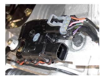
A Generation 4 Control System will typically have a build date after June 2006, and will have no external transmission range sensor. On these systems the transmission range sensor is located inside the transmission case. This application would require **Part # ILIS802-D**.
