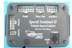
Calibration Button Fault LED
