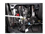
Mount the module with screws or cable ties. Ensure the module can not become loose and interfere with the driver or vehicle controls. Do not rely on double sided tape as the only method of attachment.
