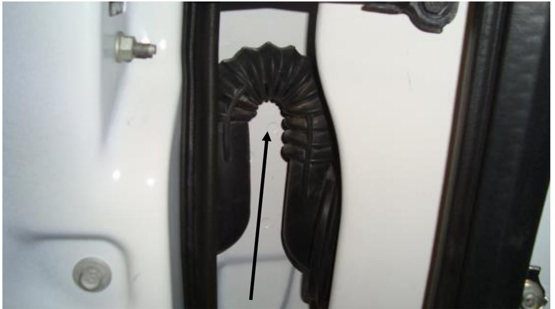
Install a grommet in the hole previously drilled in the kick panel.
