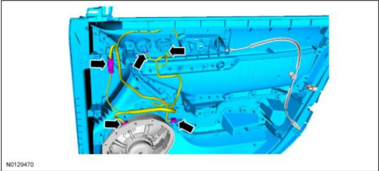
9. Release the front interior door handle cable and remove the front door trim panel.
