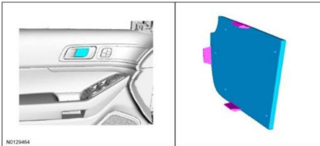
4. Using a non-marring tool, remove the front door trim panel bolt cover.
