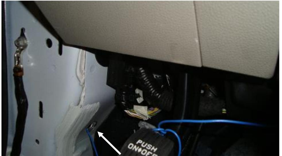
Remove the boot between the vehicle and the door and route the Gray wire through the boot and into the door panel. Removing the speaker from the door panel may be necessary.
