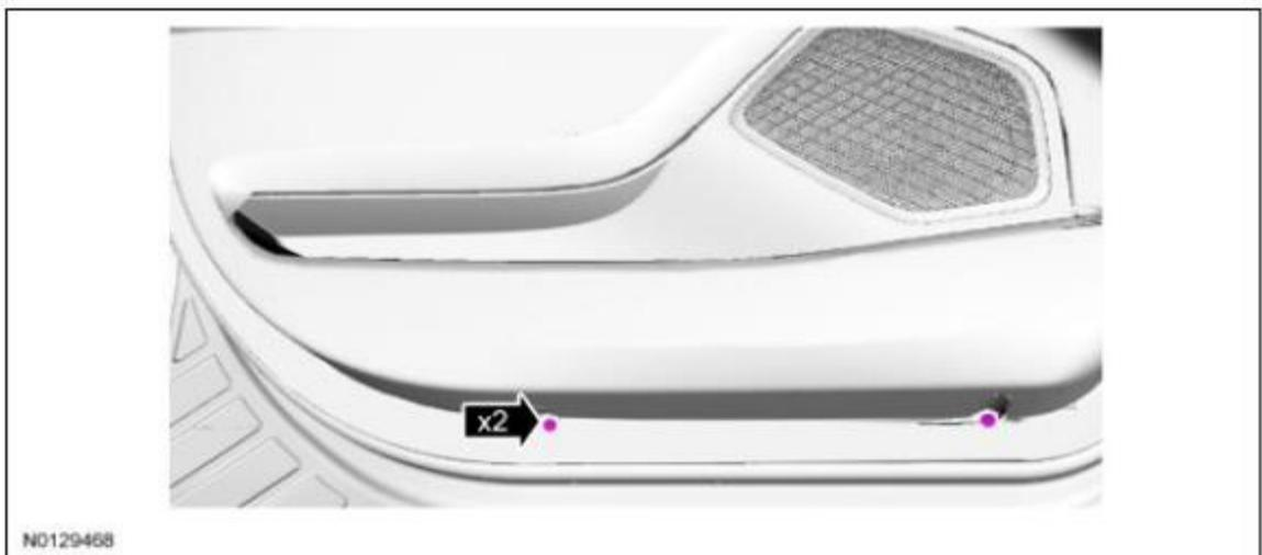
7. Using a non-marring tool, release the 8 front door trim panel clips.
