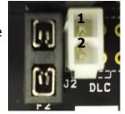
Install a 10A fuse in the fuse holder (F2) next to connector J2. Do not exceed 10A for this fuse.
