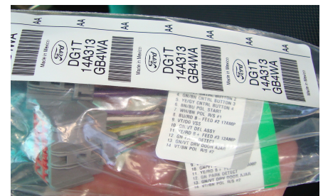
OEM provided Upfitter Harness (in glove box) mates with C2238 Connector
