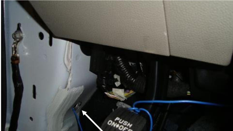
It's recommended to drill a hole in the driver's side kick panel (see photo). The hole must be large enough to accommodate a single loomed wire and a grommet. Route the Gray wire from pin 2 of the 12 pin connector through the hole.
