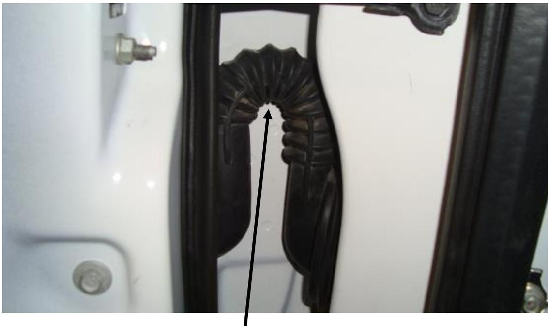
Remove the boot between the vehicle and the door and route the Gray wire through the boot and into the door panel. Removing the speaker from the door panel may make performing this step easier.
