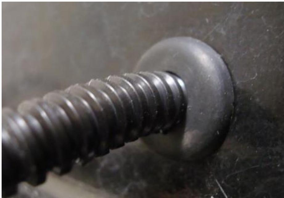
Install a grommet in the hole previously drilled in the kick panel.
