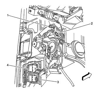
Finally, plug the orange taped 6-pin connector into the Guardian Module in the connector labeled in orange "Vehicle 1" and plug the 4-pin connector into the connector labeled in white "Vehicle 2".
