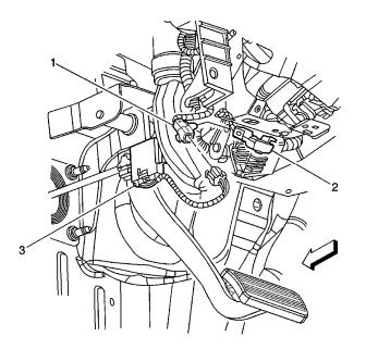
**Park Brake Connector** – Disconnect the black, single-wire Chevrolet connector from the park brake switch. Plug the female side of the Black connector from the Guardian Vehicle harness to the parking brake. (See below item 1). Install the male spade side to the female connector in the Chevrolet harness. (See below item 2).
