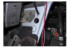
Vehicle 1 Harness connector in the two empty slots next to where the orange wire was. Either Green wire can be installed in either slot. Ensure that the metal pins securely lock into the 6-pin connector. Secure the harness with wire ties
