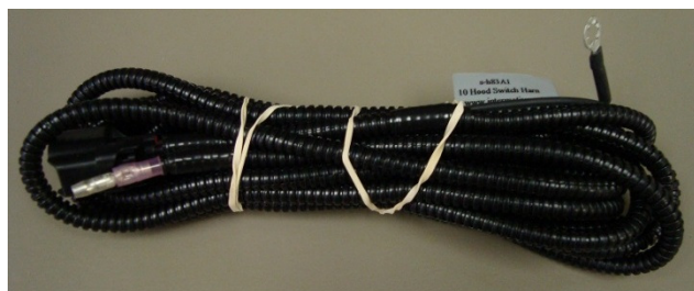
Hood switch harness—from switch to right side engine compartment & back through bulkhead. Mates with harness from module near passenger kick panel.
