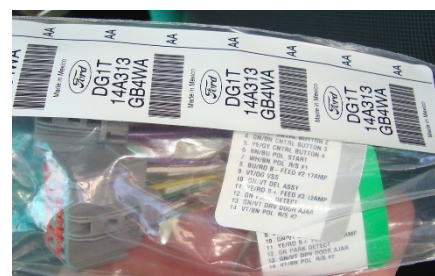
OEM provided Upfitter Harness (in glove box) mates with C2238 Connector
