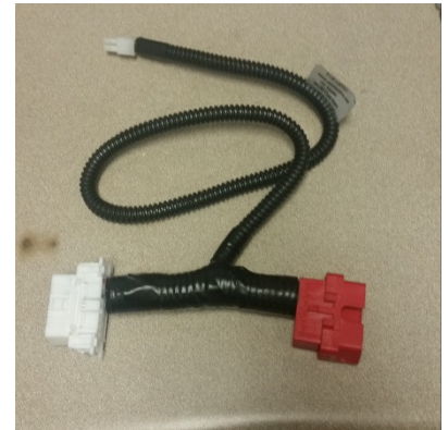
PIM Data Link harness "T's" into OBDII connector.
