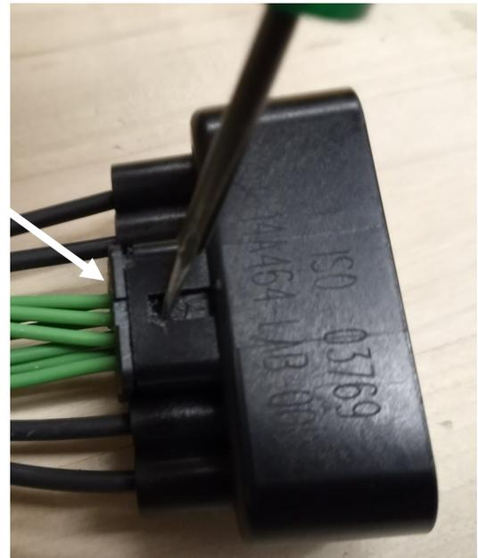
4. Pry the Blue seal from the back of the connector and slide it up the wires to the previously removed Black lock.
