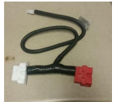
SS750 Data Link harness "T's" into OBDII connector.
