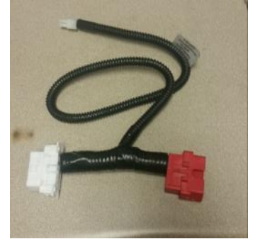
RSA Data Link harness "T's" into OBDII connector.
