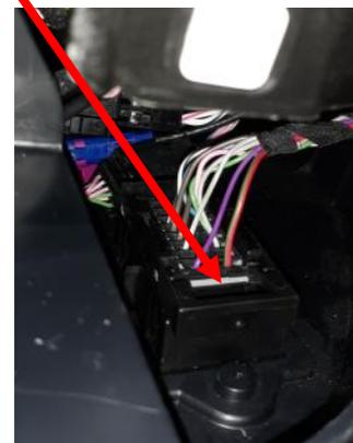
**NOTE: Do NOT plug the Data Link harness into the 6-pin connector on the PRC9xx-A module. It will be done at a later step. Do not extend the extension harness, under any circumstances.**
