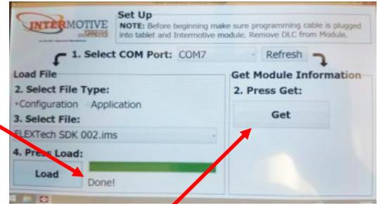
9. To verify that the correct data was loaded into the module, disconnect the 6 pin DLC connector from the module and touch the 'Get' button on the screen. "Connect DLC to Module" will come up below the 'Get' button which now says 'Cancel'.
