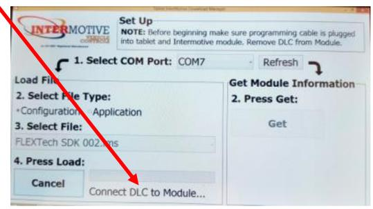
progress bar. This means the program is waiting for the power to be plugged into the PRC805/850-A module.
