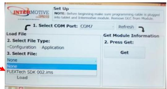
7. Touch the 'Load' button on the computer screen. "Connect DLC to Module" will come up below the
