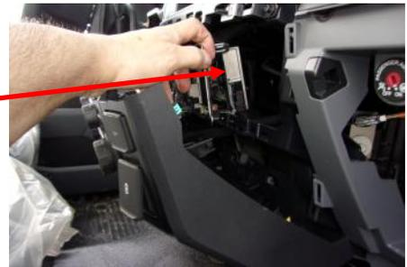
1. Remove the RH instrument panel trim using a trim removal tool. The trim starts at the ignition switch and ends at the silver clip. The glove compartment can be opened to better access the back side of the trim.
