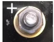
Using a calibrated torque wrench, torque the nut to 80-100 in-lbs. (Do Not Exceed 100 in-lbs) Ensure the terminal is fully seated before applying torque. After torquing, the terminal shall not rotate under light hand force. Do not exceed the maximum torque specified above. Over-torquing may result in brass thread damage, reduced electrical reliability, or PCB damage.
