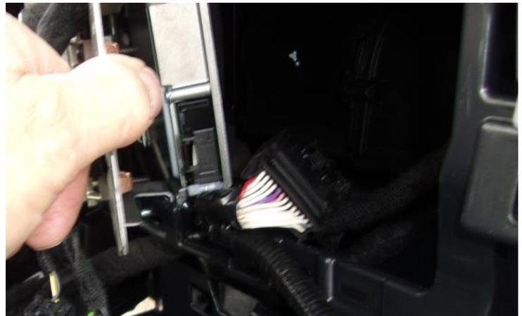
10. Run the 6-pin connector of the datalink harness to the mounting location of the module.
