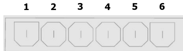
Pin Numbers for the mating connector looking from the back (wire side)
