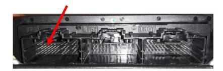
3. Unplug the Black 30-pin connector from the Gateway module and plug it into the mating connector on the PIO601 harness. Plug the male connector from the PIO601 harness into the OEM Gateway module (X1).
