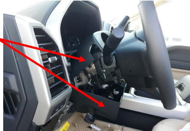
2. Locate the Shift Lock (4-pin) harness (OEM Connector 2810).
