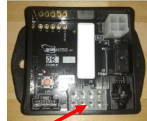
**Connect the 8 pin connector to the module**
