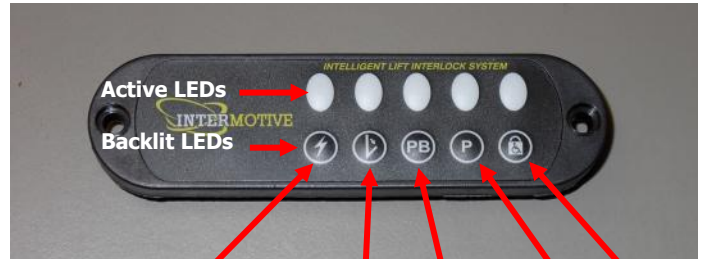
Vehicle Secure/Lift Enable, Lift Deployed, Park Brake, Park, Shift Lock
