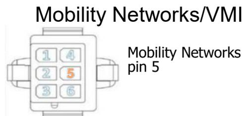
Drawings are looking into the backside of the connectors where the wires exit the connector.
