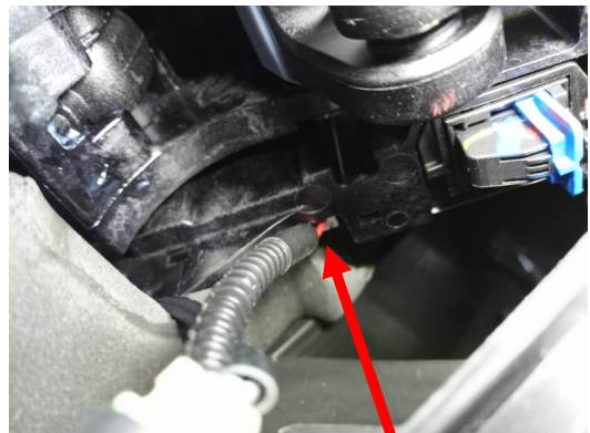
View from floor looking up at underside of transmission shifter PCB. Arrow points to the 2 pin Shift Lock Harness.
