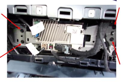
8. Disconnect the Gateway Connector by pressing down on the tab and pulling the connector away from the module.
