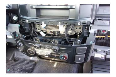
Disconnect the 2 connectors behind the center stack.
