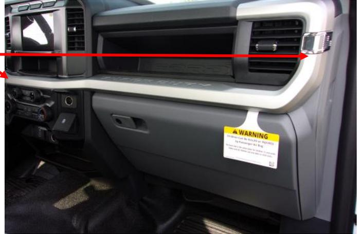
2. Using a trim removal tool, pop out the upper right corner of the lower steering column close out panel. Position it away from the center stack.
