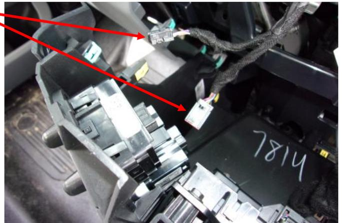
6. Detach the push-mount cable tie from the bracket and position the cable out of the way.
