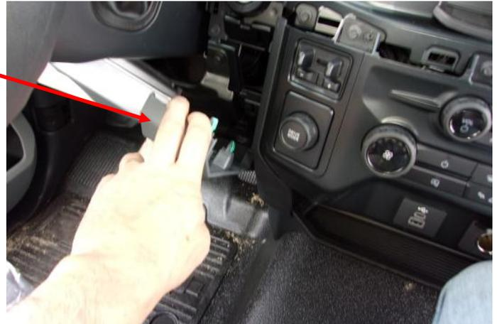
3. Remove the 4 bolts (Size: 7mm) located at the top of the center stack.
