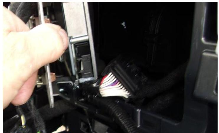
10. Run the 4-pin connector of the datalink harness to the mounting location of the module.
