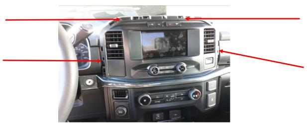
2. Remove the RH instrument panel trim using a trim removal tool. The trim starts at the ignition switch and ends at the silver clip. The glove compartment can be opened to better access the back side of the trim.
