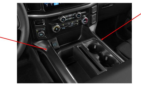
4. Remove the (4) 7 mm screws from the lower center stack trim panel.
