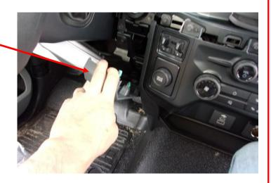
3. Remove the 4 bolts (Size: 7mm) located at the top of the center stack.
