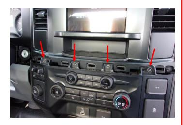
4. Release the clips on both sides of the center stack using a trim removal tool. Position the center stack away from the mounting points.
