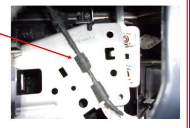
7. Remove the 4 bolts (Size: 7mm) and position the bracket away from the mounting points to access the Gateway Module. The Gateway Module is located behind the bracket.
