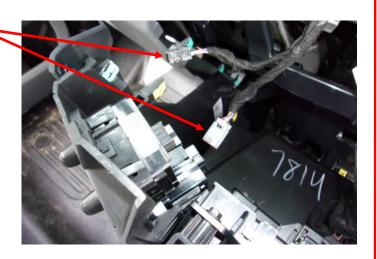
6. Detach the push-mount cable tie from the bracket and position the cable out of the way.
