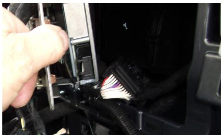
10. Run the 6-pin connector of the datalink harness to the mounting location of the AIM506 module.
