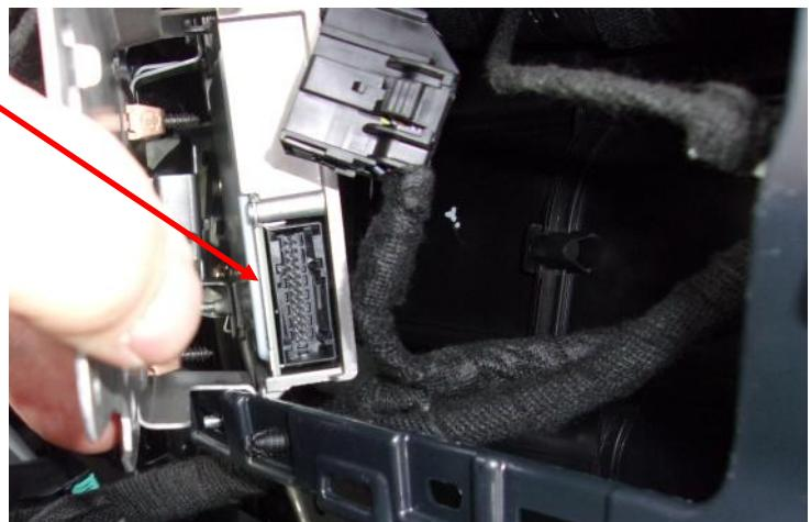
9. Install the Datalink Harness between the Gateway Module and the disconnected Gateway Connector.
