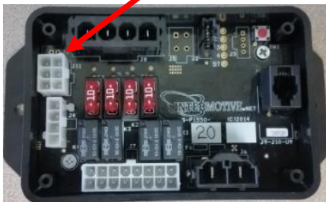
Data Link Harness plugs in here
