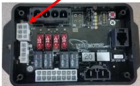
Data Link Harness plugs in here
