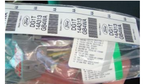
OEM provided Upfitter Harness (in glove box) mates with C2238
