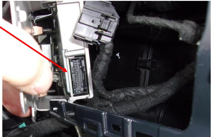
9. Install the Datalink Harness (840-00202) between the Gateway Module and the disconnected Gateway Connector.
