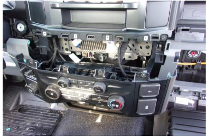
5. Disconnect the 2 connectors behind the center stack.
