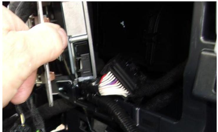
10. Run the 6-pin connector of the datalink harness (840-00202) to the mounting location of the SS502 module.
