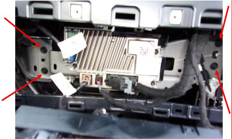
8. Disconnect the Gateway Connector by pressing down on the tab and pulling the connector away from the module.
