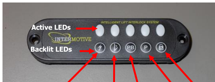
Vehicle Secure/Lift Enable, Lift Deployed, Park Brake, Park, Shift Lock
