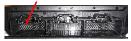
3. Remove the connector from the Gateway module, and plug it into the mating connector on 840-00179 rev 2 harness. Plug the male connector from the harness into the OEM Gateway module (X1).
