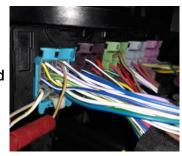
Note: Performing one step at a time, attach the correct wire to the appropriate 4-pin pigtail wire. These connections must be made using solder and the supplied heat shrink tubing. Cut the tubing to 1" lengths for this purpose.
