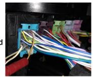
Note: Performing one step at a time, attach the correct wire to the appropriate 4-pin pigtail wire. These connections must be made using solder and the supplied heat shrink tubing. Cut the tubing to 1" lengths for this purpose.
