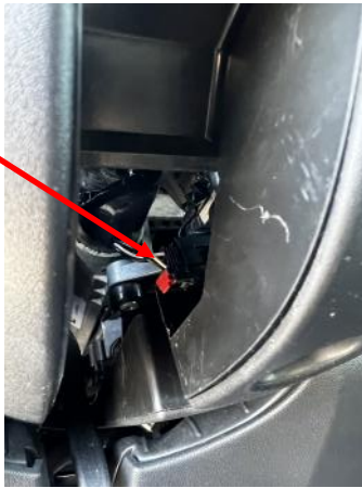
Shift Lock Connector inside steering wheel clamshell
