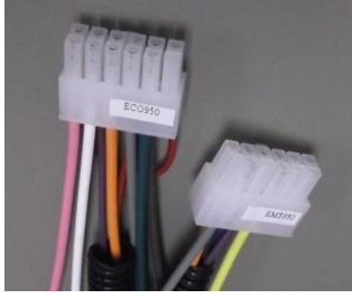
12 pin ECO and EMS connectors on ignition switch harness
