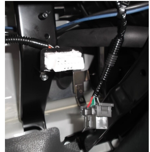
OEM OBDII bracket with White ECOEMS950 connector installed, with Grey OEM connector in lower right
