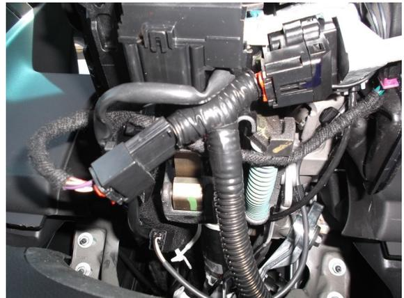
3. Plug the 12-pin and 4-pin connectors into the ECO601/602-AW module.
