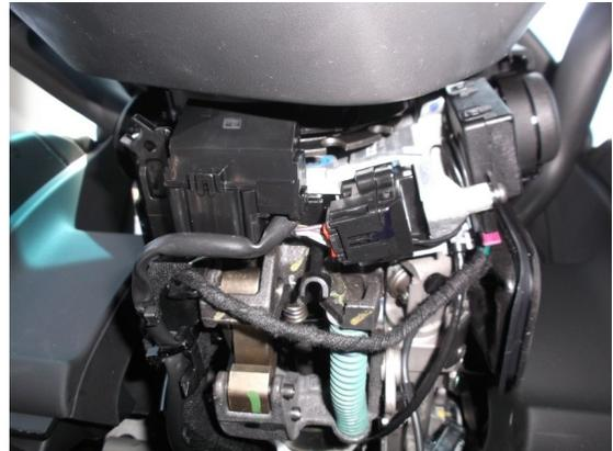
2. Remove the OEM 6 pin connector from the ignition switch and connect it to the female connector of the ECO601/602 harness. Connect the male Idle-Lock connector to the OEM ignition switch.
