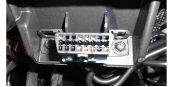
Data Link Harness plugs in here
