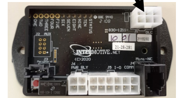
Data Link Harness plugs in here
