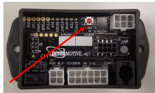
Press Test button to enter Diag Mode
